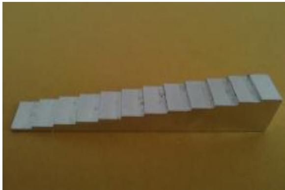
Figure 2: Aluminum step wedge
