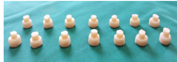
Figure 2 porcelain specimen after bonding to composite
