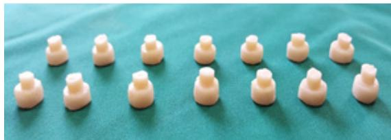
Figure 2 porcelain specimen after bonding to composite
