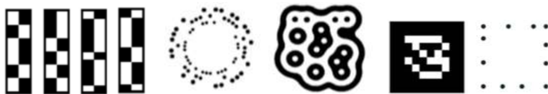
Figure 3. Photogrammetry marker code patterns in order from left to right: RID, RUNE, reacTIVision, Artag, Pi-tag (21-23). [Reproduced from: Bergamasco F et al., CVPR 2011, 2011, with permission from IEEE], [Reproduced from: Bergamasco F, Albarelli A, Torsello A, Machine Vision and Applications, 2013, with permission from Springer Science.] and [Reproduced from: Fiala M, editor, 2005 IEEE Computer Society Conference on Computer Vision and Pattern Recognition (CVPR'05), 2005, with permission from IEEE.]
