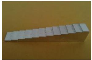
Figure 2: Aluminum step wedge
