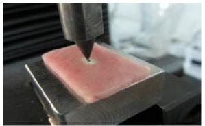
Figure.1: push-out bond strength test
