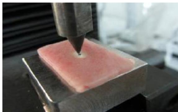
Figure.1: push-out bond strength test
