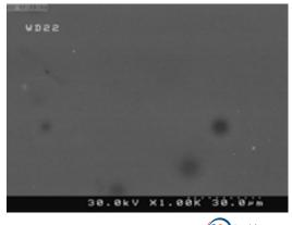
Figure 5. SEM view of zirconia
