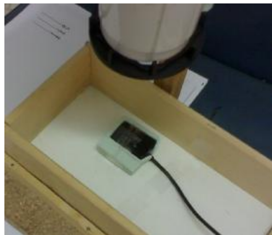
Figure 1. Prefabricated apparatus for positioning of image receptor and PID
