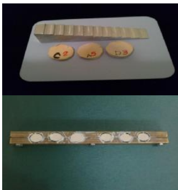
Figure 1: Step wedge and specimens in brass ring mold placed on the digital sensor
