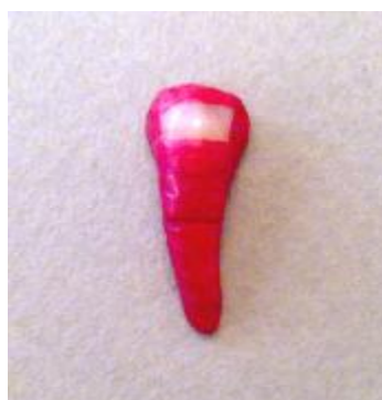
Figure 1. Divided tooth with the test area. The surrounding tooth surface was coated with nail varnish
