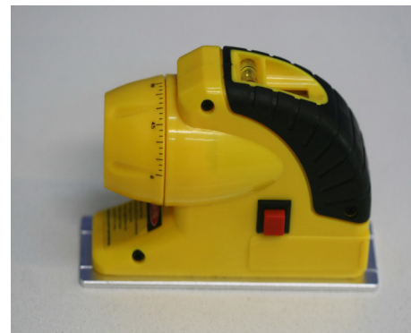
Figure 1. The laser level used for the measurement of the inclinations
